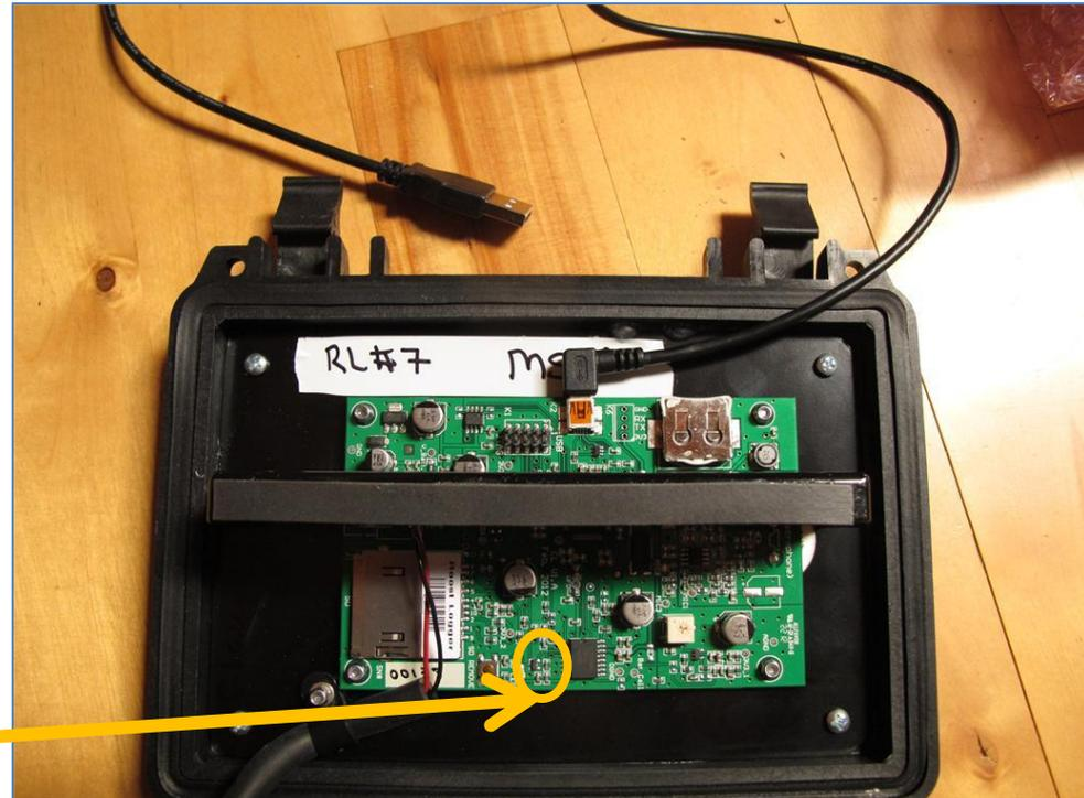
Note: this yellow light has dual purpose – it will also flash when the [SD eject button](#) is pushed for the safe ejection of the SD card.
