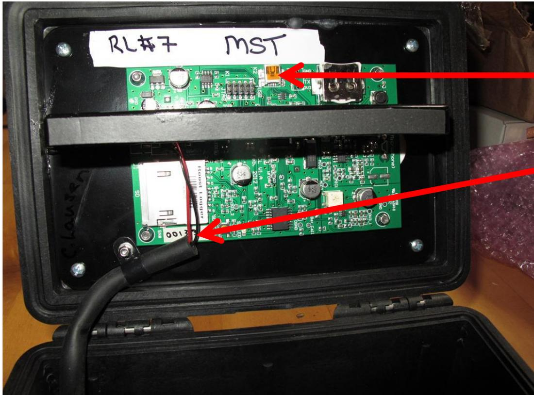
Plug for USB cable that will attach RL to computer.
